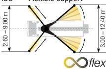
Dimensions can differ depending on configuration. Support width based on center of support leg. Diameter of swivel plate 350 mm.
