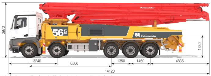
Note: Standard version. Dimensions and weights depend on truck, pump model and equipment. Dimensions in mm, MB-Actros 4640 B, Euro 2.
