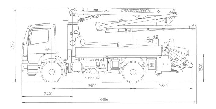
Note: Standard version. Dimensions and weights depend on truck and pump model. Dimensions in mm, MB-Axor 1523 as example
